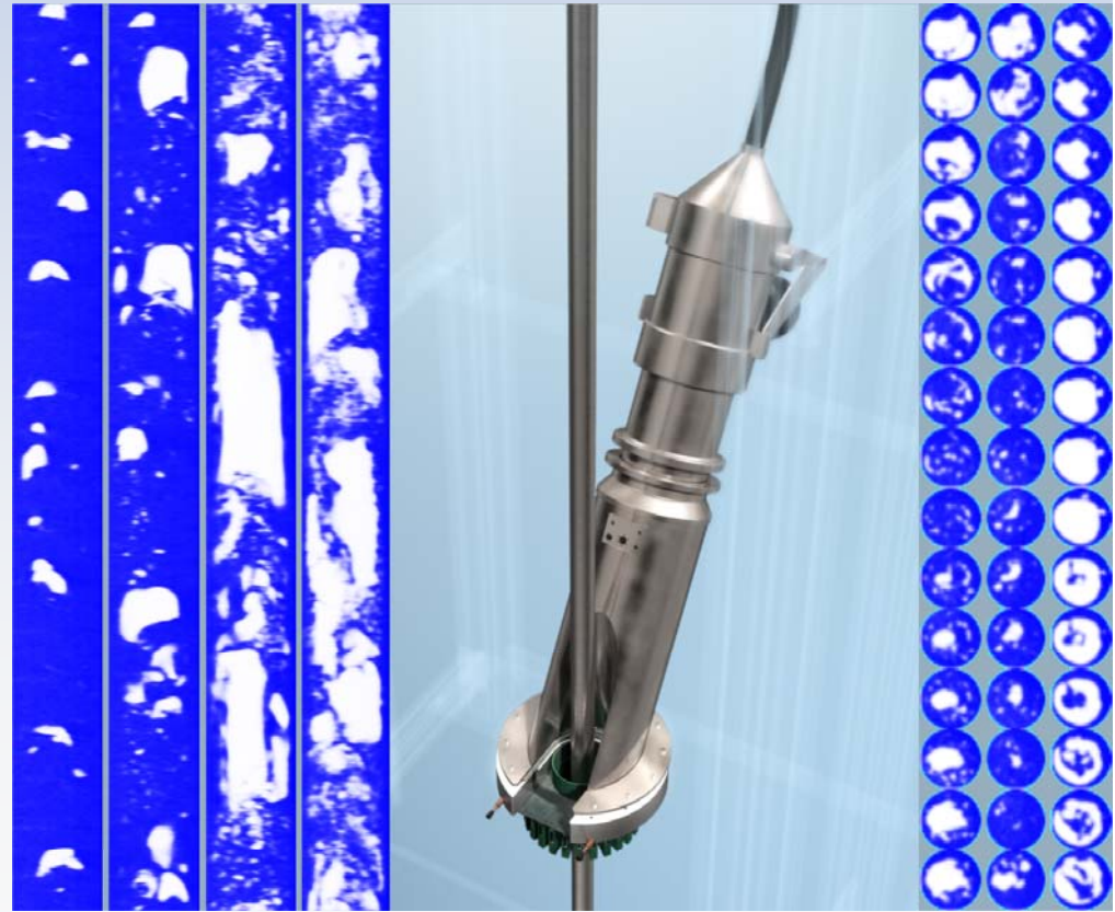
High resolution volume fraction & velocity measurements
